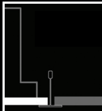
T Bar Ceiling Mounted in a T bar ceiling, without Lumafix brackets
